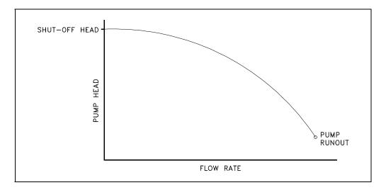
Figure 11 Centrifugal Pump Characteristic Curve
