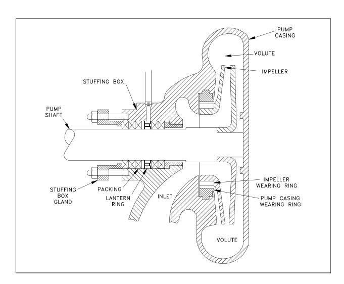
Figure 10 Centrifugal Pump Components
