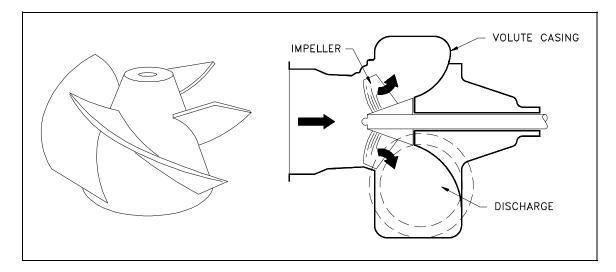
Figure 8 Mixed Flow Centrifugal Pump
