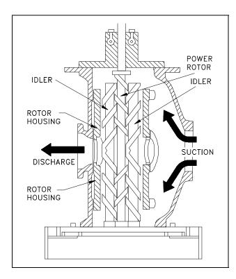
Figure 18 Three-Screw, High-Pitch, Screw Pump
