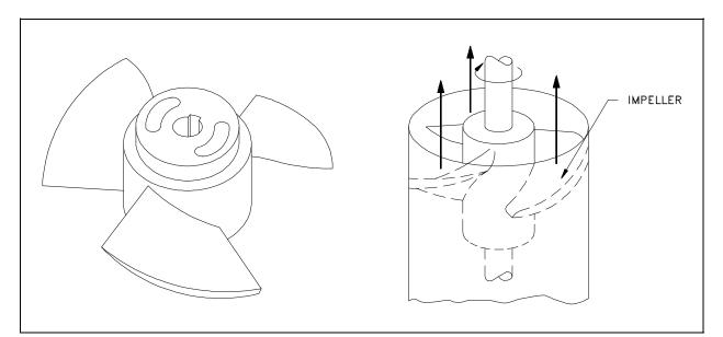
Figure 7 Axial Flow Centrifugal Pump
