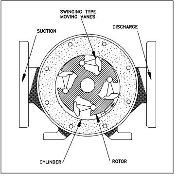
Figure 19 Rotary Moving Vane Pump
