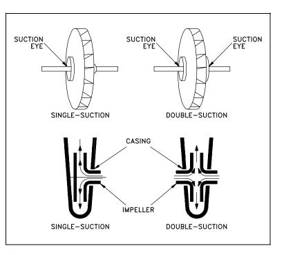
Figure 4 Single-Suction and Double-Suction Impellers
