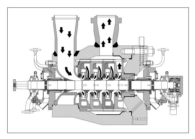
Figure 9 Multi-Stage Centrifugal Pump
