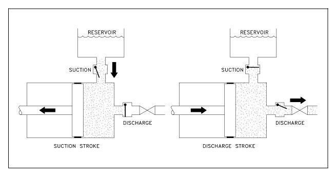
Figure 12 Reciprocating Positive Displacement Pump Operation
