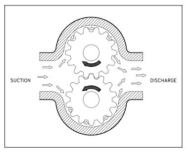
Figure 14 Simple Gear Pump
