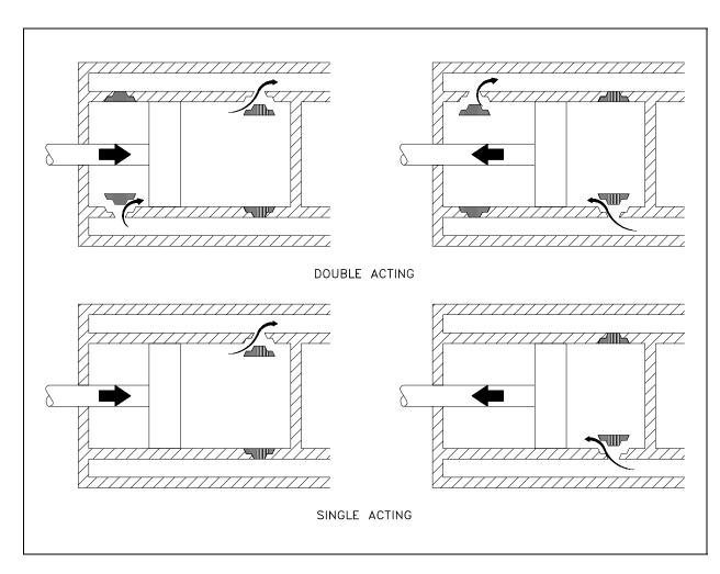
Figure 13 Single-Acting and Double-Acting Pumps
