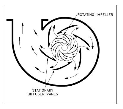
Figure 3 Centrifugal Pump Diffuser
