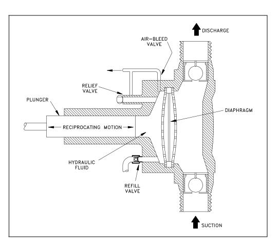
Figure 20 Diaphragm Pump
