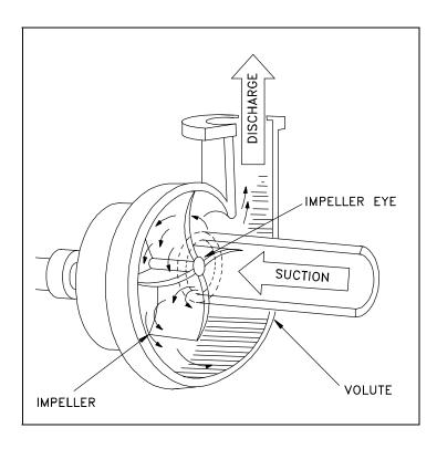
Figure 1 Centrifugal Pump
