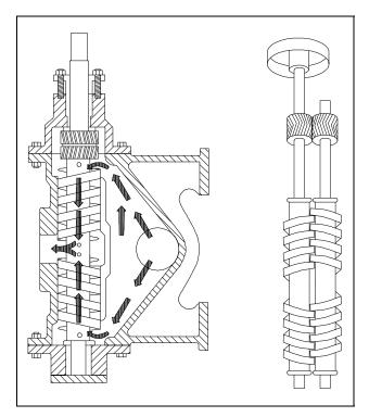
Figure 17 Two-Screw, Low-Pitch, Screw Pump
