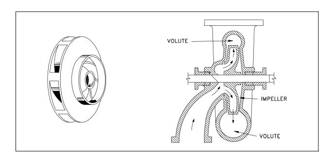
Figure 6 Radial Flow Centrifugal Pump
