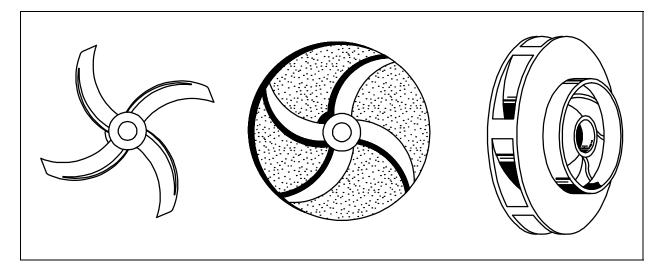
Figure 5 Open, Semi-Open, and Enclosed Impellers
