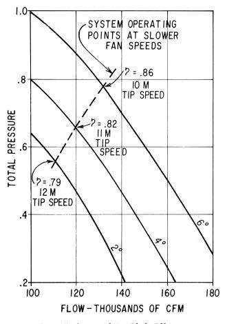
Figure 5. • ptimized Fan Blade Efficiency.
