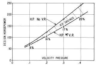
Figure 7. Effect of Velocity Recovery Stack.
