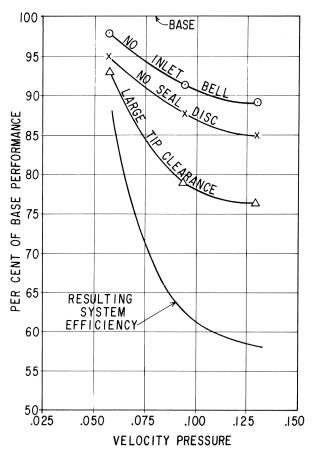
Figure 11. Results of Full Scale Fan Test.
