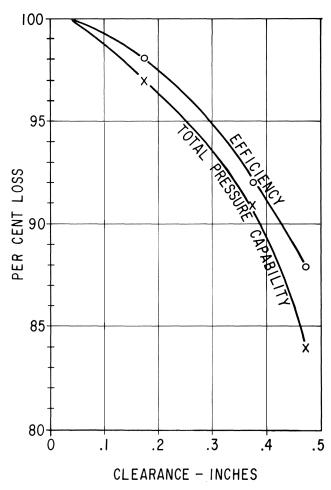
Figure 6. Effect of Tip Clearance on Small Fan.
