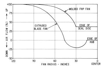
Figure 4. Results of Air Flow Test.
