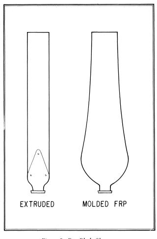
Figure 3. Fan Blade Shapes.
